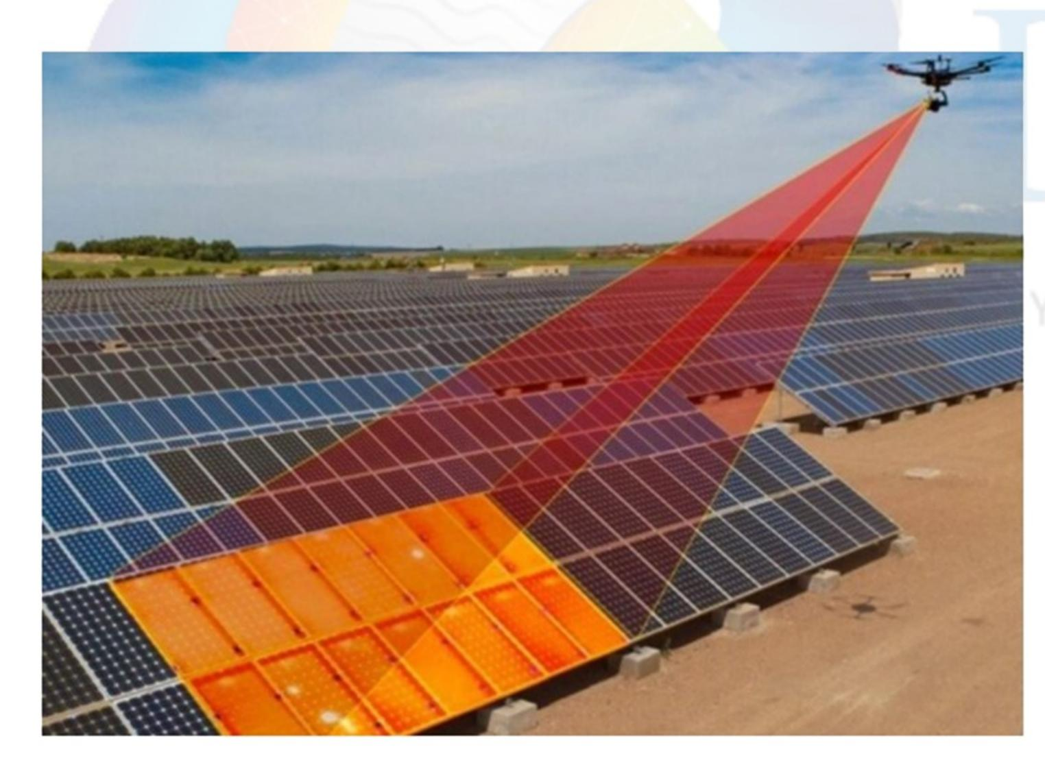
Detailed inspection of Modules using Drones fitted with Higher resolution Infrared Cameras to ascertain the following:
